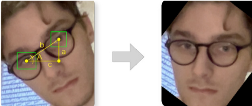
Figure 3 Face alignment by eye detection (Haar cascade method)
